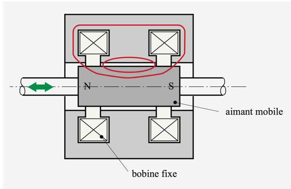
$$\vec{F}_k = \underbrace{\frac{d\lambda_{as}}{dx} \Omega_a \cdot \Omega_b}_{\text{Laplace}} + \underbrace{\frac{1}{2} \frac{d\lambda_a}{dx} \Omega_a^2}_{\text{parasite}}$$
